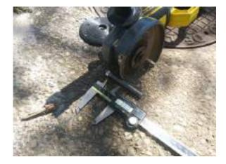
9. Cut the safety screw enough with an emery stone so that it is inserted into the socket approximately 20mm - 25mm. Take into account 5mm of extra thickness of the washer. In this case we cut to 30mm from the bottom head of the screw.
